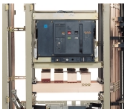
Masterpact 1600 A circuit breaker connected to Linergy busbars in a Prisma P cubicle, 600 mm depth
